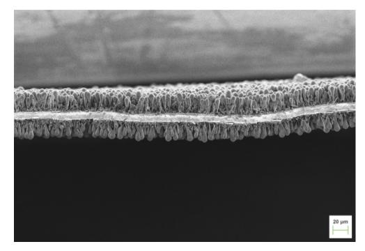
The nano-porosity of the low-density layer of silicon on each nanowire and the micro-porosity between the wires in our technology allows the silicon to expand at nano- and micro- meter levels when the anode is charged, with little to no damage to the nanowires and to the anode.
