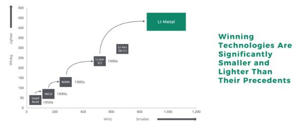
One approach to Li-Metal, known as "solid-state Li-Metal," primarily relies on solid-state materials. The solid-state material refers to the phase (solid) within which lithium ions transport from anode to cathode (during discharge) or cathode to anode (during charge). Conventional Li-ion technology uses liquid
