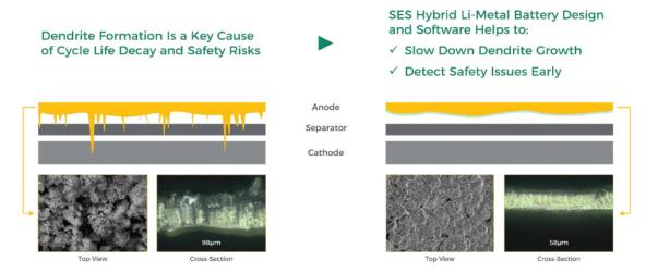
In addition to the electrolyte, our hybrid Li-Metal battery cells use a proprietary anode coating that helps provide another layer of protection against dendrites and makes lithium plating denser during charging, as well as advanced AI-powered algorithm to accurately monitor the state-of-health of the battery cells and detect any impending dendrite-related (or other) safety issues much earlier.
