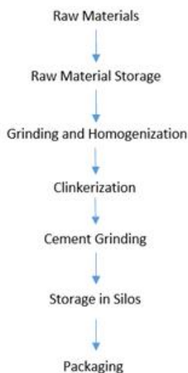
Figure 11 Pacasmayo plant process block diagram
