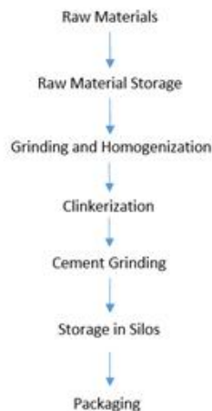
Figure 2 Pacasmayo plant process block diagram
