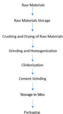
Figure 11 Rioja plant process block diagram
