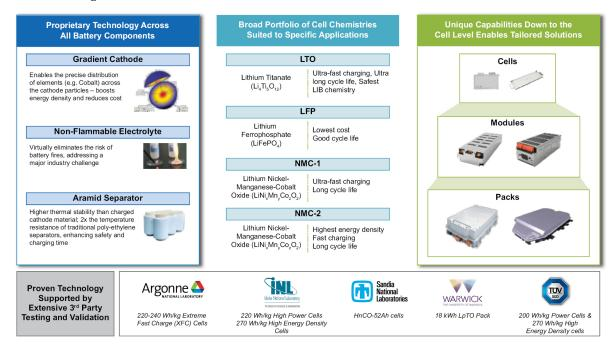
Microvast has been developing technologies for fast charging, long life, high safety batteries since the research objectives were outlined in 2008. Since then we have developed technologies spanning the battery system production through our vertical integration approach; from basic cell materials like cathode, anode and separator, to cooling systems and software controls for the battery pack. Some of the key highlights from our technology portfolio are:
