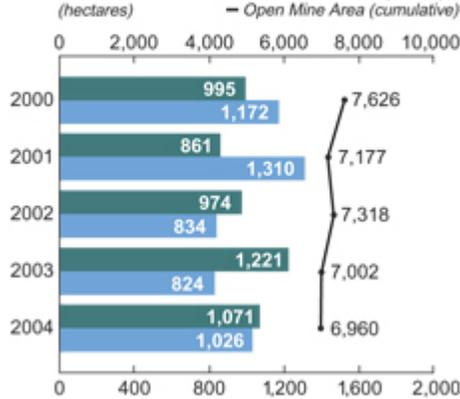
Area disturbed means annual land used in each reported year for mining or for mining infrastructure (roads, shops, crushing equipment, conveyors). Area rehabilitated means annual land returned to nature or to productive use (such as farming) after mining in each reported year. Open mine area is the cumulative area of land that has not been rehabilitated (including active mines and land used for mining infrastructure). One hectare equals approximately 2.5 acres.
