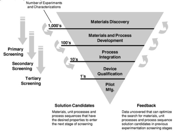
*Primary Screening.* Primary screening incorporates and focuses on materials discovery. Materials are screened for certain properties to select possible candidates for a next level of screening. In the initial primary screening there may be thousands of candidates that are subsequently reduced to hundreds of candidates.
