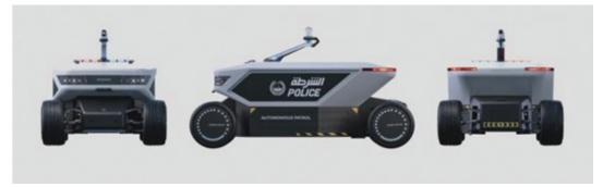
• M02: Using a similar control and drive system to M01, weighing 350KG, it offers up to 8 hours of continuous operation. Scaled to the size of a golf cart, M02 is optimized for driving within gated communities and internal roads, making it ideal for surveillance, logistics, and community utility services.
